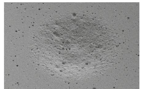
**EFFET D'UN AÉROPOLISSAGE DE 5 SECONDES SUR DU CIMENT VERRE IONOMÈR**
